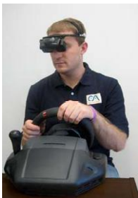
Figure 2: Tele-operation using a Head-Mounted Display
