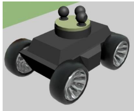
Figure 4: Wireless Cameras on top of the UGV
