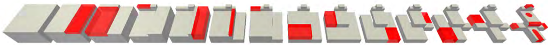
Figure 8. Examples of cutting instructions for CAD models. Some instructions steps are merged for illustration purposes.
