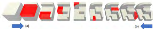
Figure 4. Cutting instructions are generated in a backward way starting from the CAD model (b). While the actual cutting is done starting from a block of material (a).
